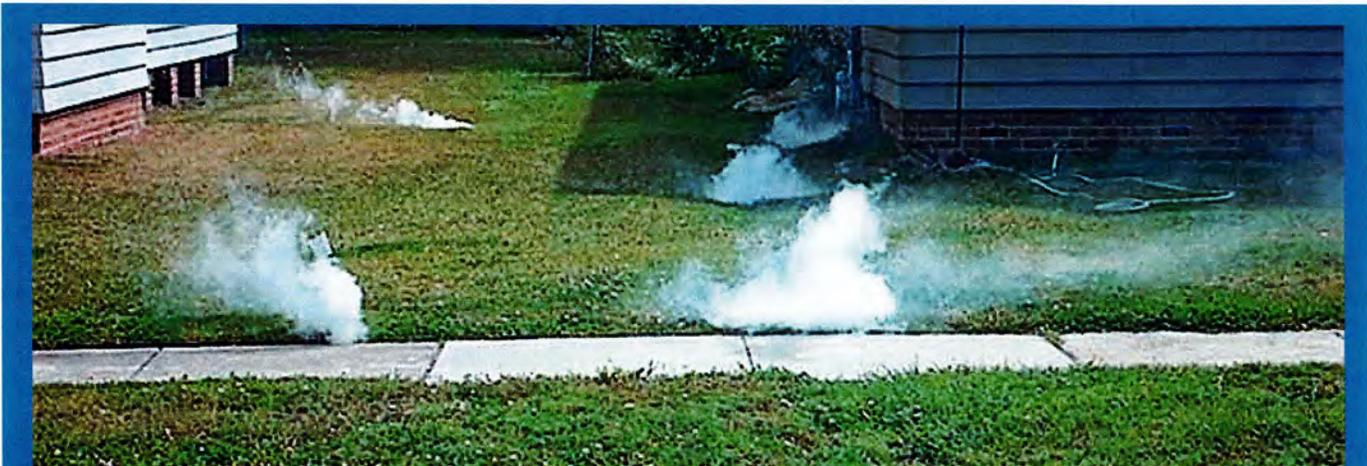
Example of smoke testing – points where water enters the sanitary system
